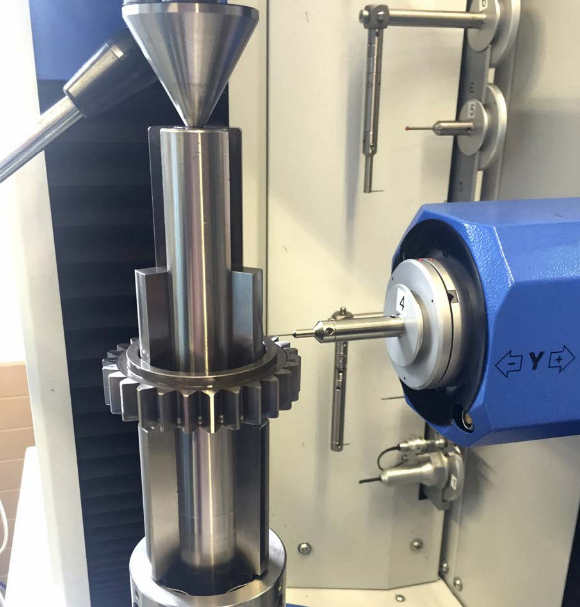
Measurement of the fully ground spur wheel clamped on the HDDS from RINGSPANN: The geometrical accuracy of the involute gearing was well within the tolerance limits! (Image: RINGSPANN)
